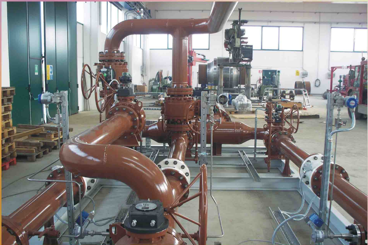
DIESEL OIL METERING SKID
